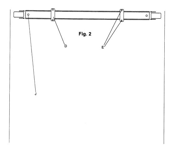
From floor to top of Mounting Bar is 30 1/2"
